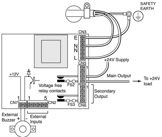
Figure 7 – Voltage Free Relay Contacts & External Buzzer Wiring
