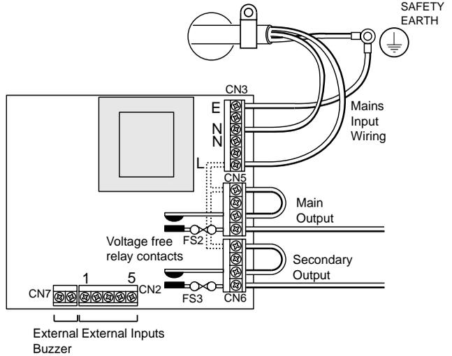
Figure 2 – Mains Wiring
