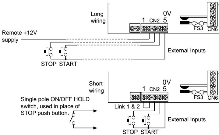
Figure 9 - External Inputs For Local and Remote Wiring
