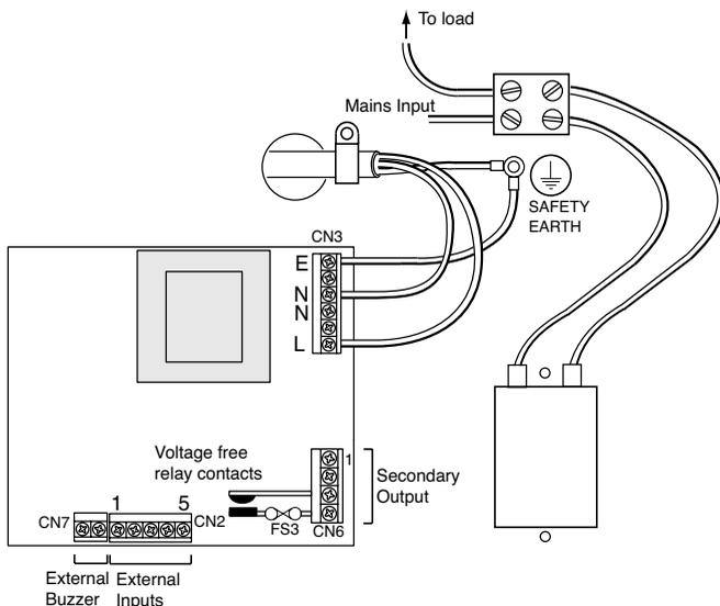
Figure 8 – 7kVA Option Wiring
