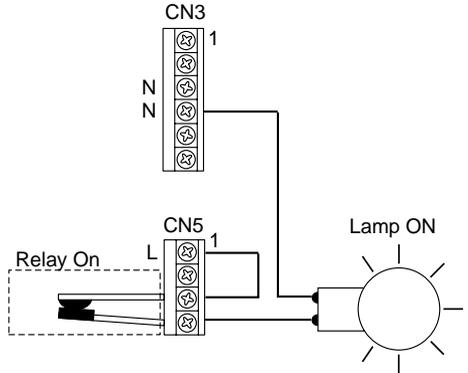
Figure 6 - CN2 and CN3 Final Wiring
