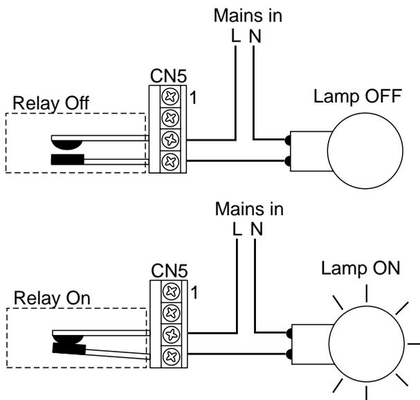
Figure 5 - Relay Contacts Wired to Control a Lamp
